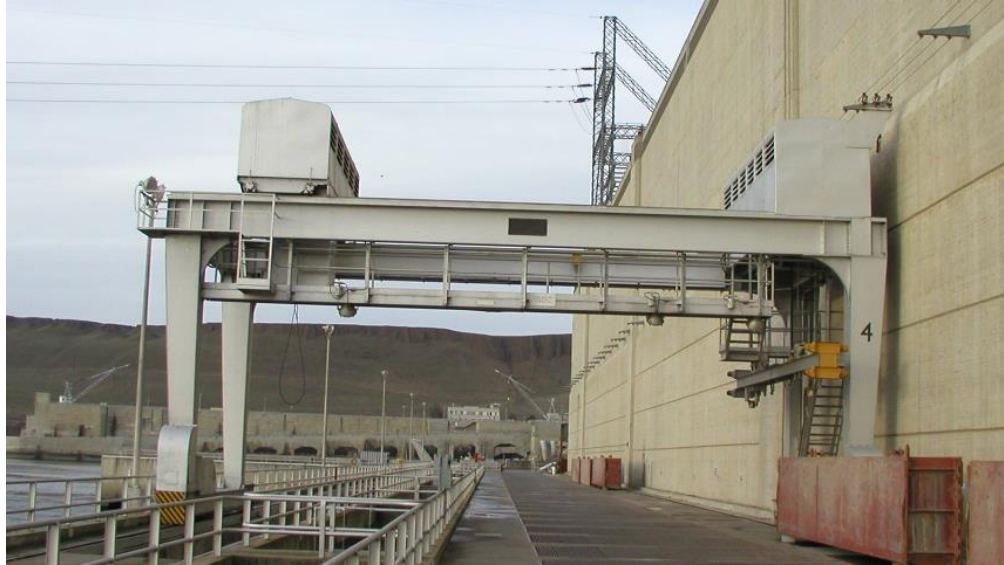
Figure 20–4. Draft tube gantry crane
