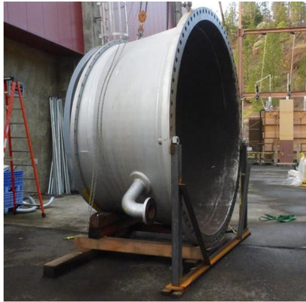
Figure 19–17. Flanged transition for valve to scroll case extension
