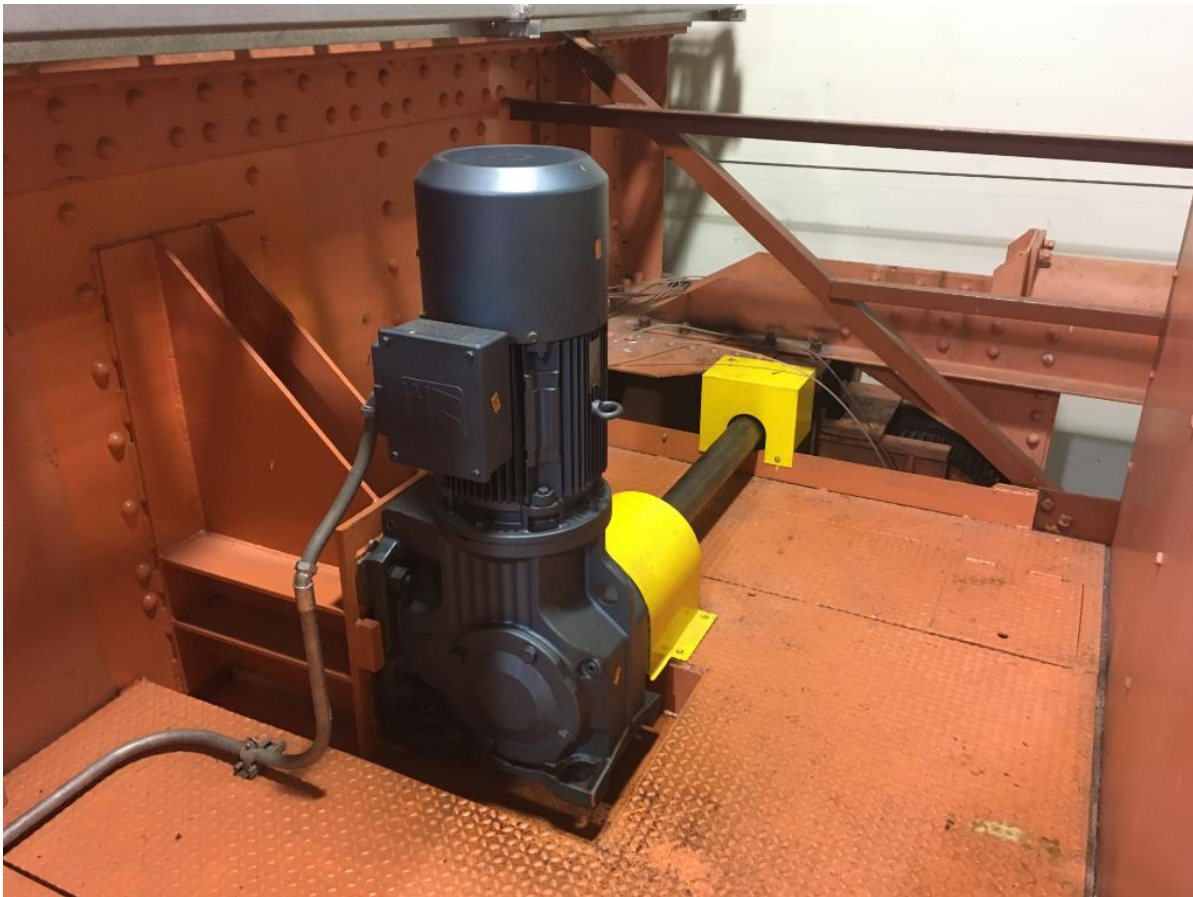
Figure 20–10. Powerhouse bridge crane with Crane Manufacturers Association of America A4 Type 1 drive arrangement
