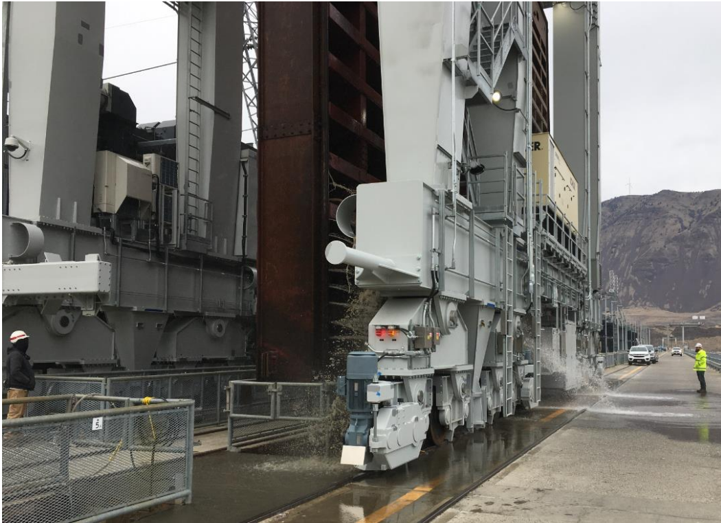
Figure 20–7. Powerhouse gantry crane with Crane Manufacturers Association of America A4 drive arrangement
