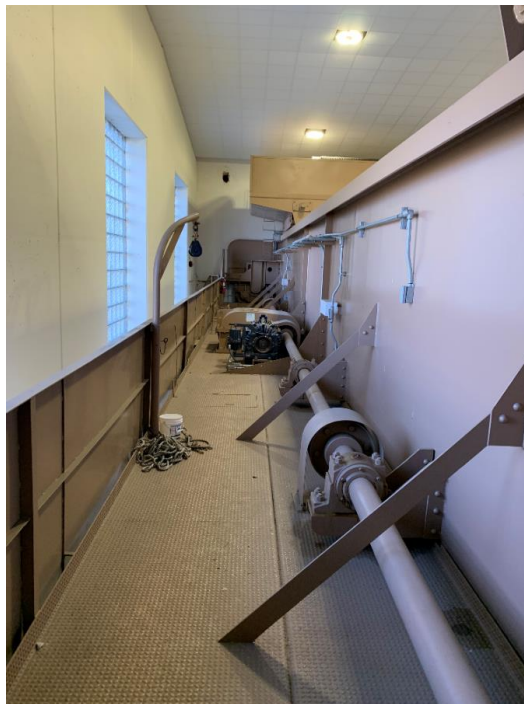
Figure 20–8. Powerhouse bridge crane with Crane Manufacturers Association of America A1 drive arrangement
