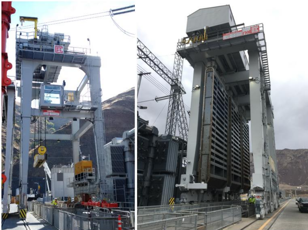
Figure 20-3. Intake gantry crane (left) and emergency intake gantry crane (right)
