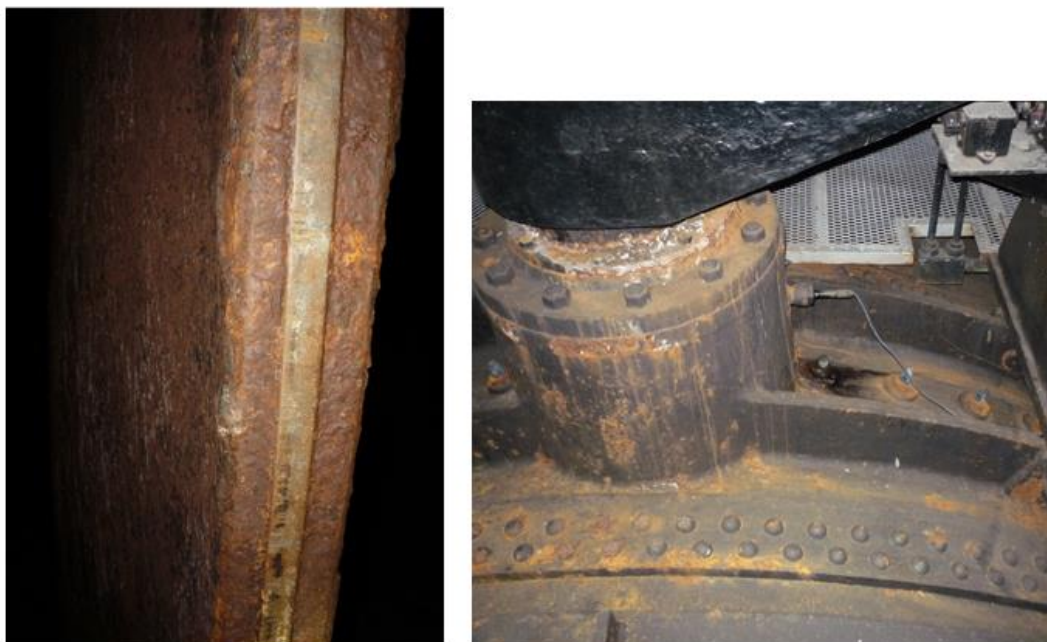
Figure 19–24. Valve disk (left) and valve body surface corrosion and operational damage
